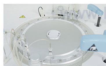
Reaction Tray 37±0.1°C, water bath
