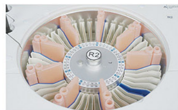
Reagent Tray 2~8°C cooling for 24 hours.
